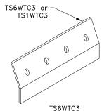
bare metal thickness (t) = 0.0538 in. (1.37mm)
